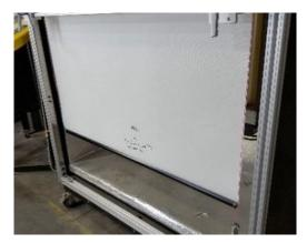
Image 10: Fiberglass Core Fabric in Heatbox
