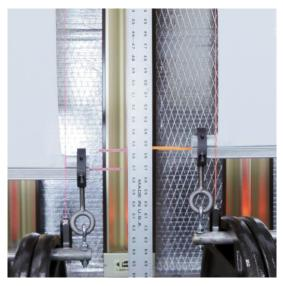
Image 15: Heated Elongation Comparison (6hr) Polyester (left), Fiberglass (Right)
