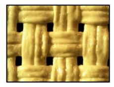
Image 3: Fiberglass Core Fabric Surface (80x)
