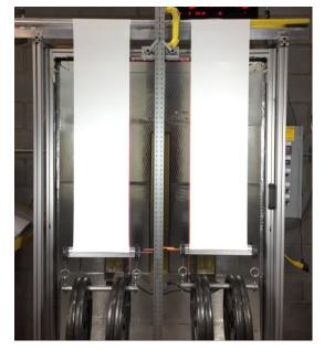
Image 12: Weighted Elongation (Room Temp-24hr) Polyester (left), Fiberglass (Right)
