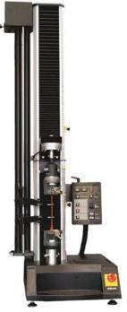
Image 7: Single Column Tensile Tester
