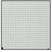
Image 5: Fiberglass Core Fabric Surface (1.0 in<sup>2</sup>)
