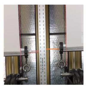
Image 14: Weighted Elongation Comparison (24hr) Polyester (left), Fiberglass (Right)
