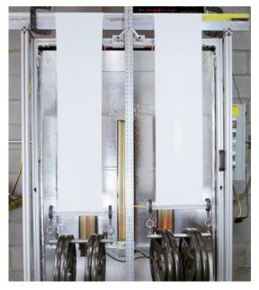
Image 13: Heated Elongation (140°F-1hr) Polyester (left), Fiberglass (Right)
