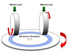
Image 9: Taber Abrasion Test Diagram (ASTM D3884)
